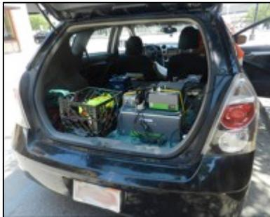
The Picarro CRDS installed in the car
